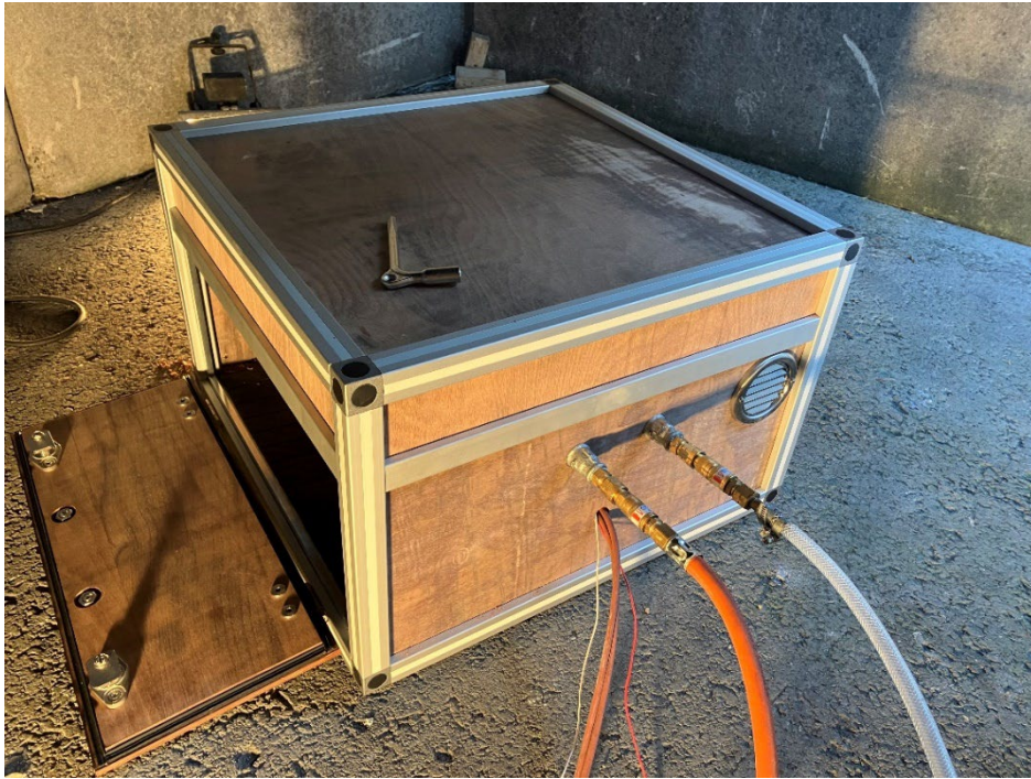
Figure 1: External view with gas and compressed air connection and cable feedthrough for the fan
